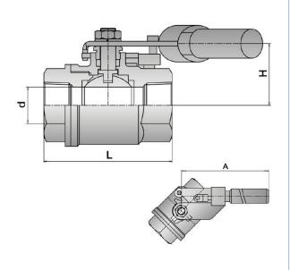
Connection 1: G 3/8" Material: 1.4408 PN: 130 DN: 10 G: G 3/8" d: 12,5 L: 57,0 H: 29,5 A: 184 Weight: 540 g
