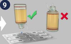
Keep the bottle inverted in case any additional drops may be required. If the bottle has been turned upright at any stage of this process it is important to return to step 5
