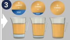
Agitate sample using a swirling motion and leave to settle for 12-15 mins. Once settled, check that there is free water present to conduct a test
