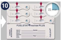
Leave the FUELSTAT° test plate on a flat surface for 10-15 minutes. A dark red line 'Control line' should appear on the left-hand side of each of the 6 viewing windows. This indicates that the test has worked correctly
