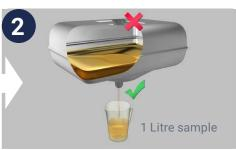
Take a 1 Litre sample from the lowest point in the tank ensuring bottom water is collected following OEM and industry guidelines (sampling advice on page 1)
