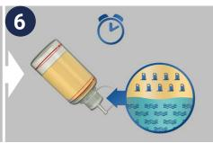
Invert test bottle 45° and allow the blue fluid to settle out in the shoulder of the bottle. NOTE: for a free water phase only test the blue fluid will not separate out
