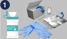
Clean sample equipment using 70% alcohol wipes and let dry. Have the FUELSTAT® test kit contents at hand. Wear correct PPE, including Nitrile gloves and safety eyewear when handling fuel.
