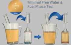
If there is visible free water but not enough to reach the 'Water line' when syringed into the FUELSTAT® test bottle, continue syringing fuel from near the bottom of the sample up to the top line marked 'Fuel line'
